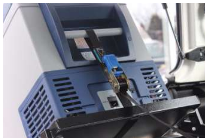
Figure 6: Ratchet strapped fridge.
