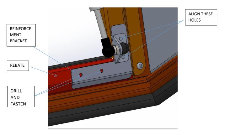
Remove the lower gas strut mount by drilling out the rivets. Align the reinforcement bracket holes and fasten with bolts and nuts. The nut should be on the inside of the canopy. Mark and drill the two holes at the bottom of the rebate and fit fasteners.
