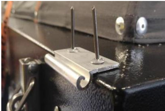
Figure 6: Rivets in 38mm Extrusion Alu
