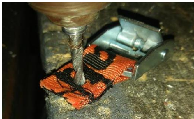
Figure 10: Drilling the hole into the buckle
