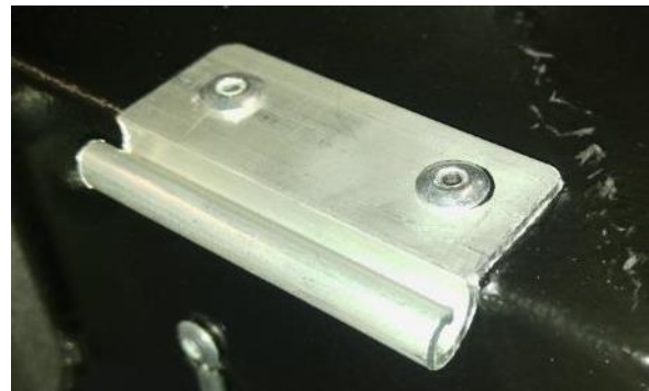
Figure 7: 38mm Extrusion Alu riveted in place
