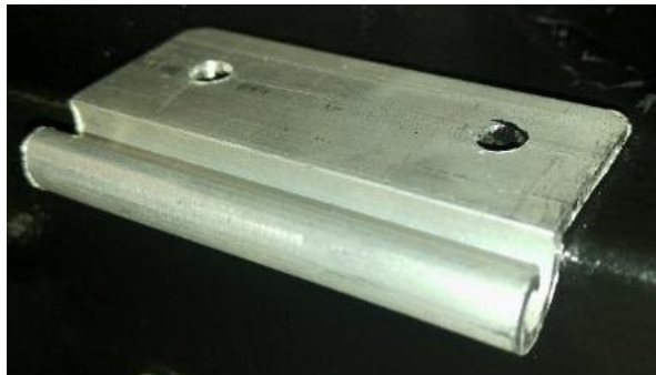
Figure 5: 38mm Extrusion Alu with holes drilled into
