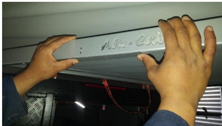
Figure 15: Black Adhesive foam strip attached
