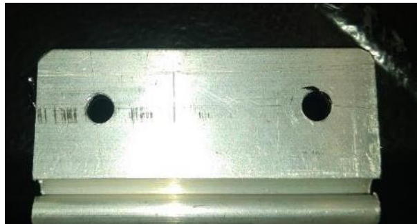
Figure 4: 38mm Extrusion Aluminium with holes drilled
