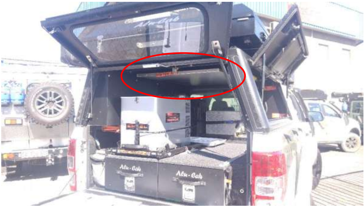
Figure 12: Table fitted into canopy (Outside photo)
