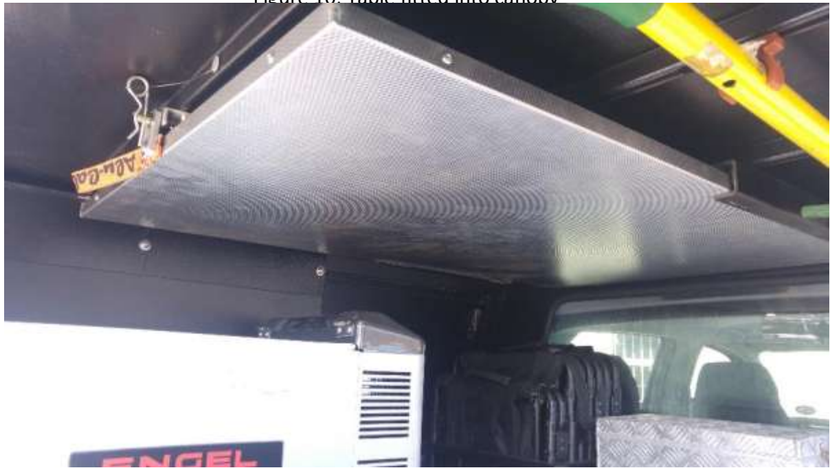
Figure 11: Table fitted into canopy (Inside view)
