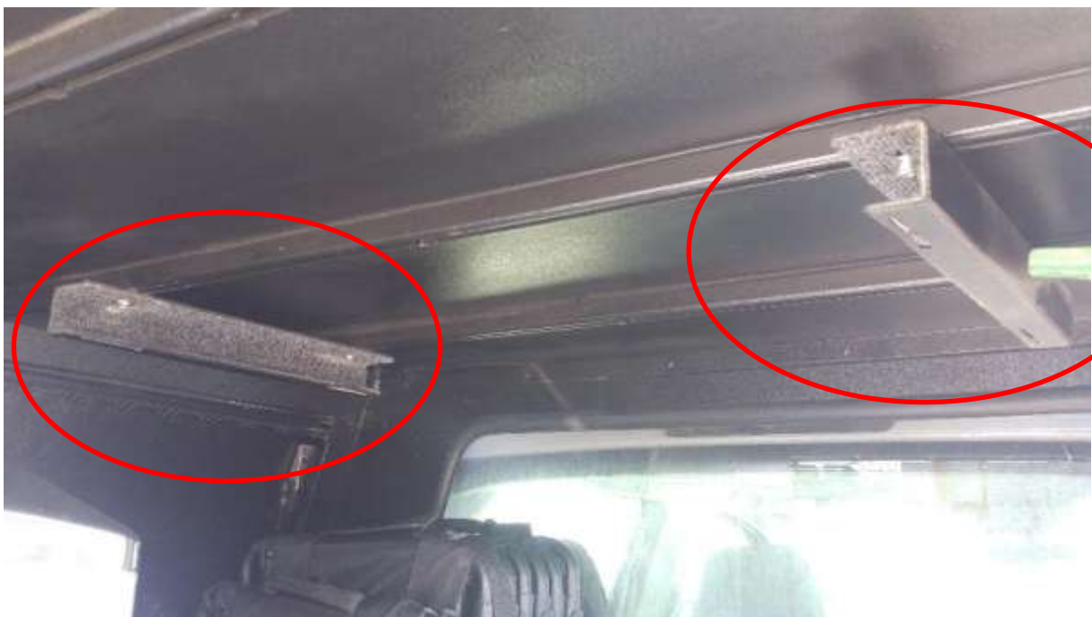
Figure 3: Table brackets installed
